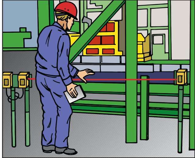
Regular functional testing of safety installations.
